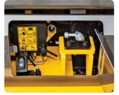
**Cabin Tilting Automatic System** Cabin tilting automatic system makes servicing of all power train components quick and easy. An electrically assisted hydraulic actuated cylinder tilts operator cabin to left side about 53 degrees for easy access to inside of truck components.
