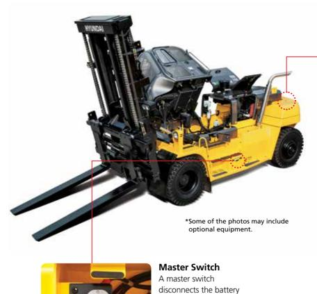
power to protect the electrical system from excess electrical drainage.
